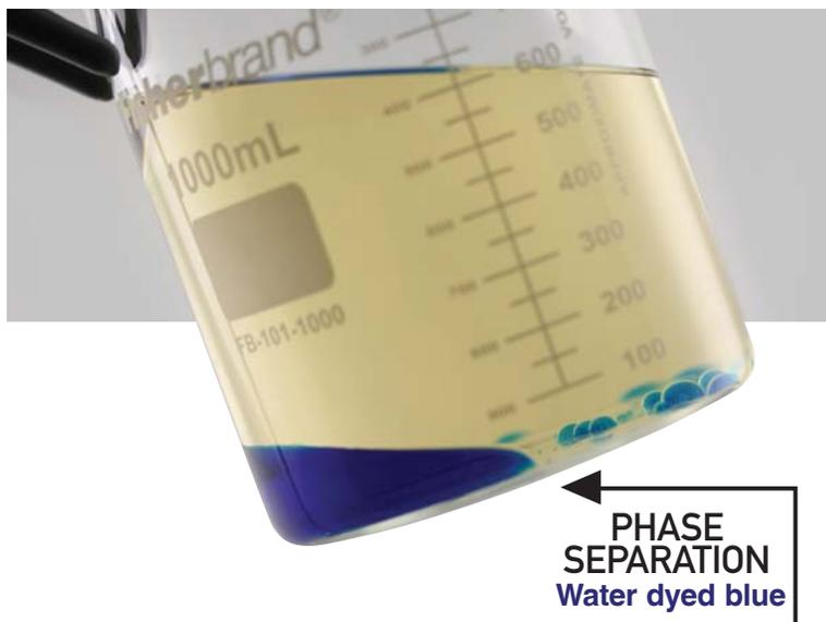
When ethanol/water mixtures fall to the bottom of fuel containers, it leads to lean-burn situations. Quickshot helps keep water molecules dispersed to prevent phase separation.
